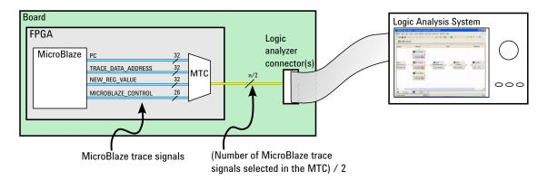
In addition to the signals shown here, there are four additional status signals and a clock signal.
