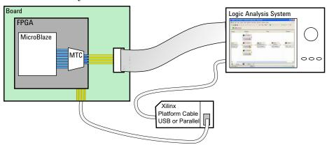
The connector must match the logic analyzer probe you plan to use. Examples of such connectors include MICTOR, Samtec, and pads for an Agilent soft touch or pro-series soft touch connectorless probe.
