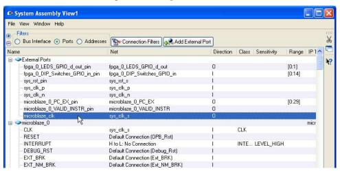
6 Modify your UCF file. Add pin locations for the MicroBlaze trace outputs as shown in the example below. Note that the actual pin locations are user-defined. (This example shows PC\_EX for MicroBlaze4; for MicroBlaze5, this bus bus is called PC).
